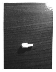
The Ink cartridge is then grappled and connected to the upper portion of the pen through the plastic connector. The connector is the part of the pen that is attached to the end of the ink cartridge and is the direct link that connects it to the piston. Without this mechanism, the contents inside the pen would not feel any tension too keep the other parts up right and in line. This part is more of a connecting piece, as its name implies, yet it is still an important piece that
